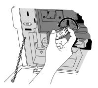
4 Locate the development unit release lever. Move the lever clockwise until it locks into place.
